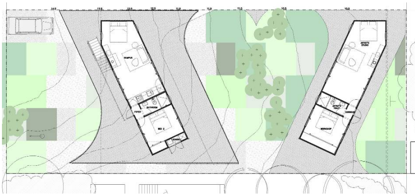
Figure 8 Plan showing 2 levels of units with large communal deck and detached studio.
