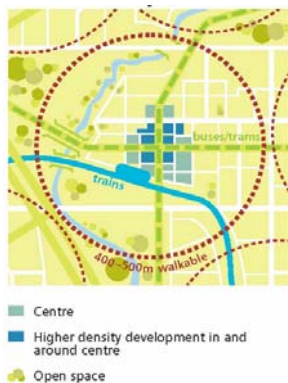
Figure 7, Diagram from Melbourne 2030 (2003) showing five minutes walking distance catchment measured from centre of transport interchanges.
