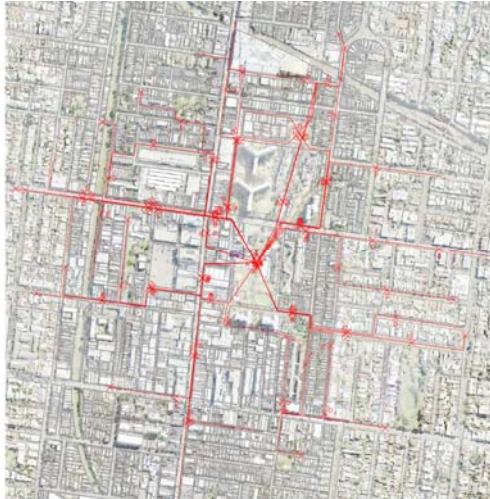
Figure 8. AutoCAD drawing with aerial photo background showing possible routes from chosen node in Red. These routes are polylines with total length of 800m.
