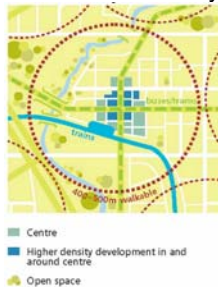
Figure 2, Diagram from Melbourne 2030 Planning for Sustainable Growth (2003), showing five minutes walking distance catchment measured from centre of transport interchanges.
